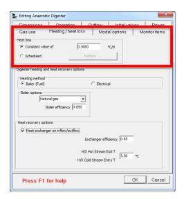
The heating power requirement is provided from a fuel or electrical source [see later], but there are also options in BioWin for heating power recovery within the Anaerobic Digester and Thermal Hydrolysis Unit elements. *The heat recovery option for anaerobic digesters is a new BioWin 5.2 feature*:
