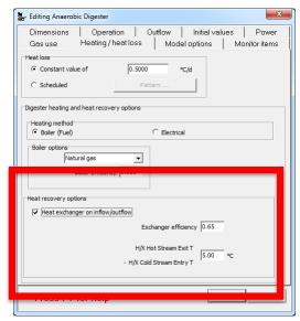
When the option to include a heat exchanger is specified, BioWin assumes that the hot digester (or THU) output stream is used to heat the cool incoming stream in a counter-current heat exchanger. Users can enter the efficiency of the exchanger as well as the temperature difference between the heat exchanger's hot exit stream and cold entry stream. A schematic representing the difference in temperature between the hot exit and cold entry streams for the heat exchanger is shown below.
