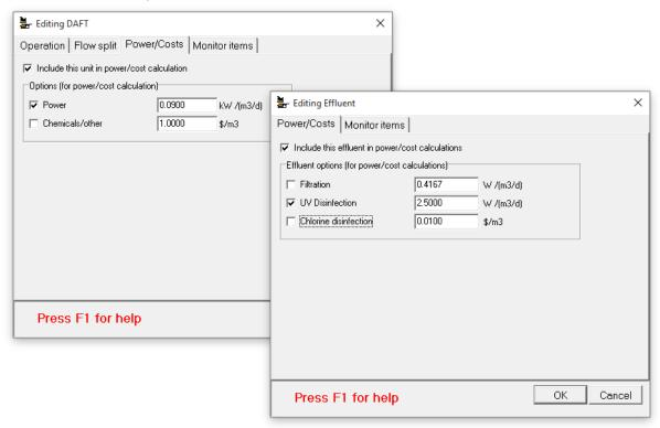
In BioWin 5.2, all elements can track power demand on either a unit volume/flow basis, or a direct user-input kW (or hp) basis. Each of these options can be constant, or vary with time as shown below:
