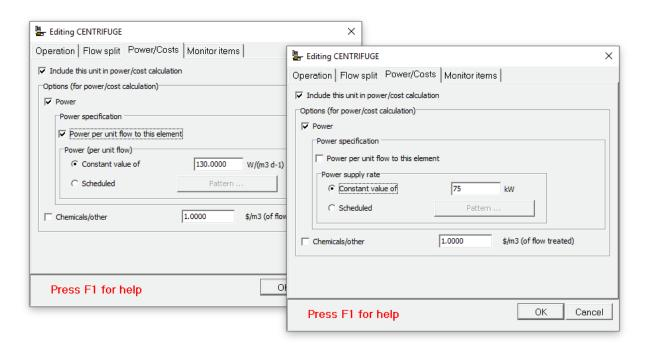
Additionally, sludge output elements now have the ability to track power demand on either a unit flow basis, or a direct user-input kW basis (*neither option was available for sludge output elements in BioWin 5.0*). This allows for tracking of energy requirements for certain sludge disposal technologies.
