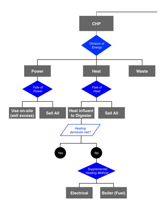
2. Burning the biogas in a boiler for heating and supplementing *via* electrical or external fuel sources if insufficient gas is available. If there is any excess biogas after satisfying heating demands, there is an option to sell it.
